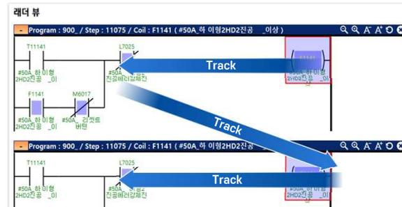
Analyze past signal paths to determine failure causes and highlight the end control contact in the logic flow.
